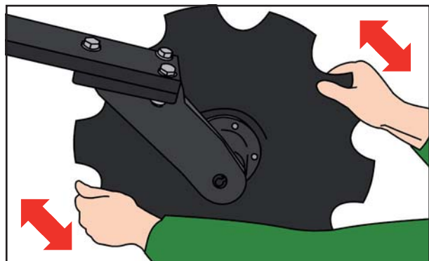
Fig. 5.01: Checking Disc Bearing Adjustment
