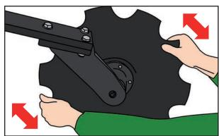
Fig. 5.01: Checking Disc Bearing Adjustment
