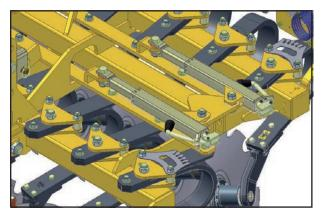
Fig. 4.05: Disc Angle Adjustment Jacks
